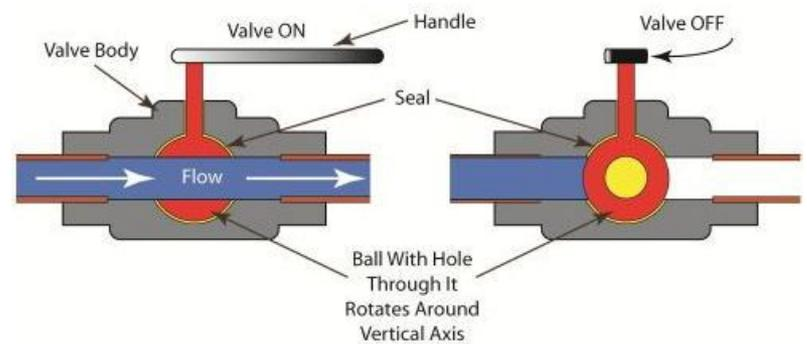
Advantages. A ball valve is generally the least expensive of any valve configuration and has low maintenance costs. In addition to quick, quarter turn on-off operation, ball valves are compact, require no lubrication, and give tight sealing with low torque.
