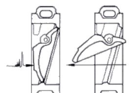
The general types of check valves are swing, tilting-disk, piston, butterfly, and stop.
