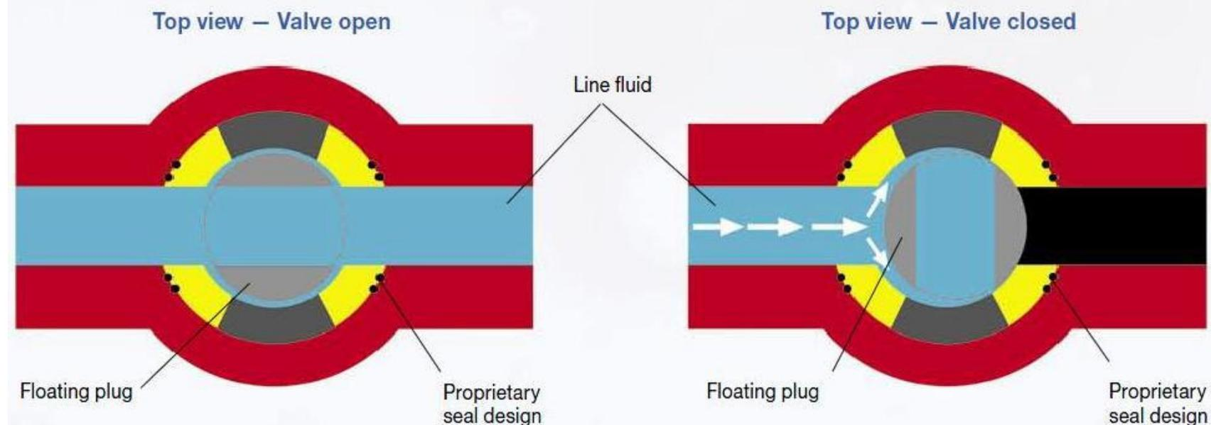
Plug valves are available in either a lubricated or non-lubricated design and with a variety of styles of port openings through the plug as well as a number of plug designs.
