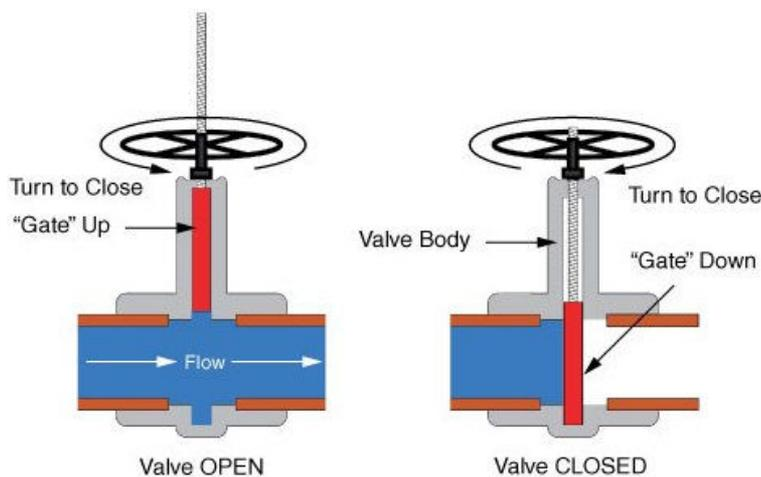
A gate valve can be used for a wide variety of fluids and provides a tight seal when closed. The major disadvantages to the use of a gate valve are:
