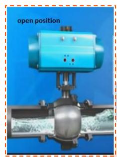
outlet side. In an open position, the flow is allowed across the pipeline and in the closed position the flow stops.
