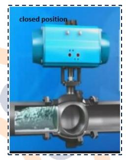
Actuators in shutdown valve There are many valve actuators available, but there is something which we should consider deciding which one is suitable for the shutdown valve and for the preparation of the process system. As the function of SDV for emergency needs the actuator must be able to close the valve quickly i.e. the standard timing is 3 secs. We must explain to the vendor that they must make calculations for
